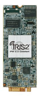
IPMI 2.0 adapter card with 2620 BMC chip for IEI IRIS2 Connector IPMI 2.0 module
