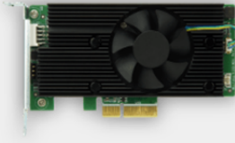
Mustang-V100-MX4 4 x Intel® Movidius™ Myriad™ X MA2485 VPU Accelerator
