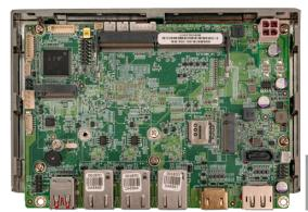
3.5" SBC with Intel® 10nm Jasper Lake Celeron® N5105 Processor with Dual Displays, DDR4, Triple Intel® 2.5 GbE, USB3.2, M.2, SATA, COM, SoC, RoHS
