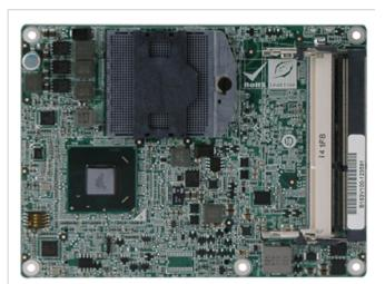
COM Express Basic Type 6 Module with Socket G2 Supports Intel® 2nd &3RD Generation Core™ i7/i5/i3 Celeron® Processor
