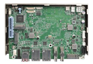
3.5" SBC supports Intel® Celeron® J6412 on-board SoC, triple display with DP, HDMI™ and IDPM slot, dual 2.5 GbE, USB 3.2 Gen 2, M.2, SATA 6Gb/s, COM, iAUDIO and RoHS, -10°C ~60°C
