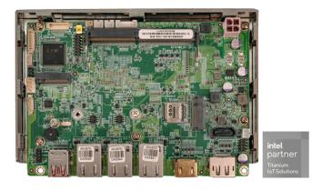
3.5" SBC with Intel® 10nm Jasper Lake Celeron® N5105 Processor with Dual Displays, DDR4, Triple Intel® 2.5 GbE, USB3.2, M.2, SATA, COM, SoC, RoHS
