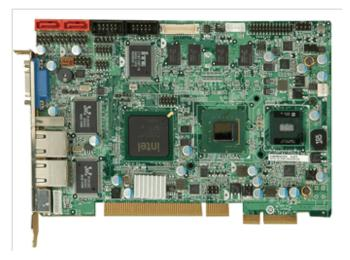
Half-size PCIe CPU Card with Intel® Atom™ Processor
