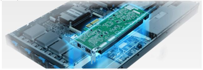
NVMe drive bays of PUZZLE-9030 support PCIe Gen4 x4 channel which provides up to 7000MB/s data transmission speed. It is 2 times faster than PCIe 3.0 U.2 (3200MB/s) and 10 times faster than SATA (500MB/s).
