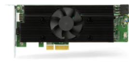
IEI Mustang-V100-MX8 Accelerator with 8 Intel® Movidius™ Myriad™ X MA2485 VPUs
