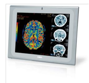
19" Medical Panel PC features Intel® Core™ i7/i5/i3 mobile processorwith Intel® HM55 chipset
