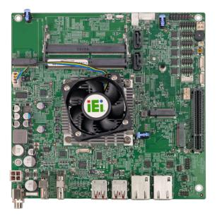
Thin Mini-ITX SBC supports Intel® Tiger Lake-UP3 Processor, 9 ~ 36V DC input, triple independent displays, HDMI™, DP, iDPM, SATA 6Gb/s, Dual Intel® 2.5GbE, USB 3.2 Gen2, M.2 and RoHS
