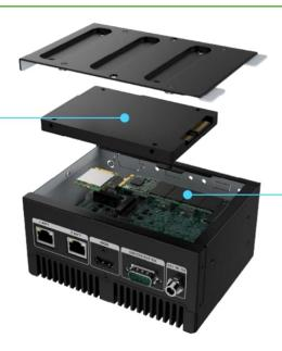
M.2 M-key slot for NVMe SSD (via PCle Gen3 x2)
