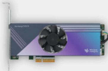
Mustang-T100-T5 5 x Google Coral edge TPU Accelerator
