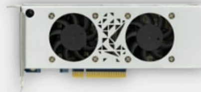
Mustang-F100 Intel® Arria® 10 GX1150 FPGA Accelerator
