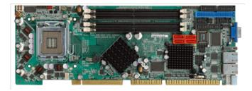
Full-size PICMG 1.0 CPU Card supports LGA 775 Intel® Core ™2 Duo, Pentium® D, Pentium® 4 and Celeron® D Processors
