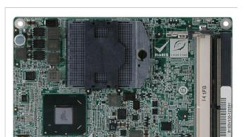
COM Express Basic Type 6 Module with Socket G2 Supports Intel® 2nd &3RD Generation Core™ i7/i5/i3 Celeron® Processor
