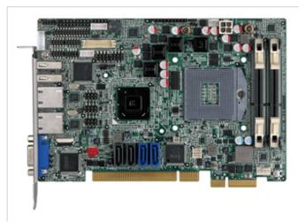
Half-size PCIe CPU Card supports Socket 988B Intel® Mobile Core™ i7/i5/i3 or Celeron® CPU with Intel® HM65
