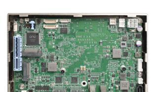
3.5" SBC supports Intel® Celeron® J6412 on-board SoC, triple display with DP, HDMI™ and IDPM slot, dual 2.5 GbE, USB 3.2 Gen 2, M.2, SATA 6Gb/s, COM, iAUDIO and RoHS, -10°C ~60°C
