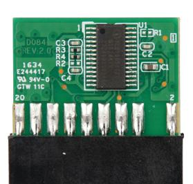
Hardware-based security solution for data protection and reliable authentication via TPM that stores key, passwords and digital certificates.
