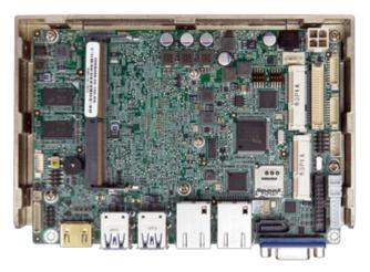
3.5" SBC supports Intel® 7th Generation ULT Processor with DDR4 SO-DIMM/On-board Memory Support
