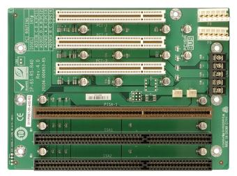
6-slot backplane with three PCI slots and two ISA slots
