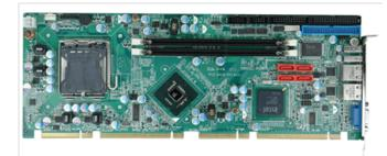
Full-size PICMG 1.3 CPU Card supports LGA 775 Intel® Core ™2 Quad Processor
