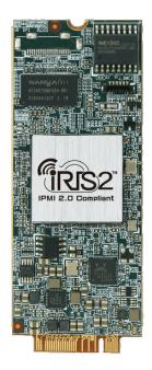
IPMI 2.0 adapter card with 2620 BMC chip for IEI IRIS2 Connector IPMI 2.0 module
