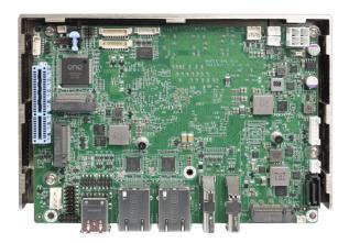
3.5" SBC supports Intel® Celeron® J6412 on-board SoC, triple display with DP, HDMI and IDPM slot, dual 2.5 GbE, USB 3.2 Gen 2, M.2, SATA 6Gb/s, COM, iAUDIO and RoHS, 0°C ~60°C
