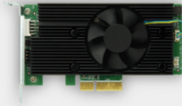
Mustang-V100-MX4 4 x Intel® Movidius™ Myriad™ X MA2485 VPU Accelerator
