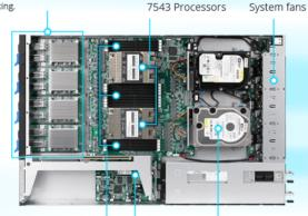
16-slot 8-channel DDR4 RDIMM/LRDIMM
