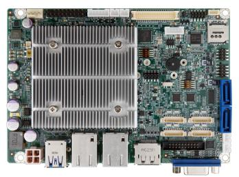
3.5" SBC supports Intel® 14nm Generation Atom ™ or Celeron® on-board SoC with DP++/VGA/LVDS/iDP support
