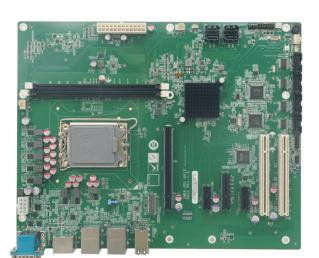
ATX motherboard supports LGA1700 Intel® 12th/13th Generation Core™ i9/i7/i5/i3, Pentium® and Celeron® processor, DDR4, Triple independent displays, 2.5GbE LAN, USB 3.2, SATA 6Gb/s and RoHS
