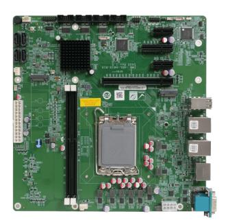
micro ATX motherboard supports LGA1700 Intel® 12th/13th Generation Core™ i9/i7/i5/i3, Pentium® and Celeron® processor, DDR4, Triple independent displays, dual LAN, USB 3.2, SATA 6Gb/s and RoHS
