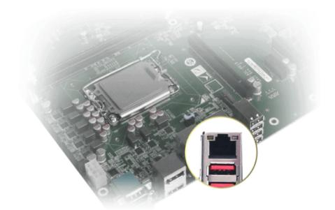
Delivers Low-Latency 2.5G LAN Powered by Intel The on-board Intel® I225V 2.5GbE controller enable the IMBA-ADL-H610 to meet the bandwidth-intensive requirements such as large file transfers and high-resolution video streaming applications.
