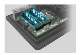
Compared to a SATA SSD drive, an NVMe-based drive can write to disk up to 2x faster. Thus, the NVMe system is a great solution to enable applications that require real-time data processing and analysis, such as autonomous vehicles, machine learning, surveillance and industrial automation.
