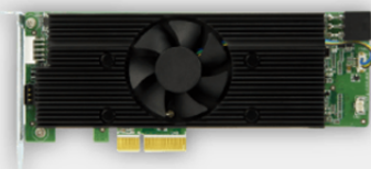
Mustang-V100-MX8 8 x Intel® Movidius™ Myriad™ X MA2485 VPU Accelerator
